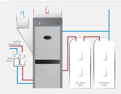
During the heating cycle, the fluid circulates through the loop extracting heat from the ground. The heat energy is transferred to the geothermal unit. The unit compresses the extracted heat to a high temperature and delivers it to your home through a normal duct system or radiant heat system.
